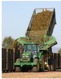
*Figure 2 Haul-out unit loading a cane bin*
